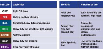
Buffing pads are lightest in color and remove scuff marks and dirt. It brings a semi-gloss back to the wax. Used at 175 - 600 RPM.
